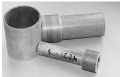
Fig. 4. Technological wastes after hot pressing and drawing of Al-W-B prepregs.
