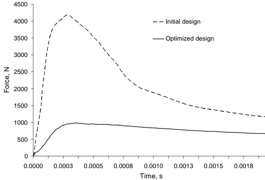
**Fig. 5.** Force–time diagram: initial design and the optimized design.
