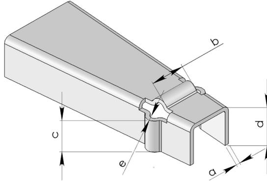
Fig. 2. Energy absorbing component ( $a$ ,  $b$ ,  $c$ ,  $d$  and  $e$  are design variables).
