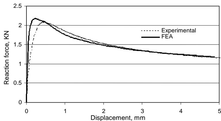
Fig. 4. Load–displacement curves: experimental and FEA.
