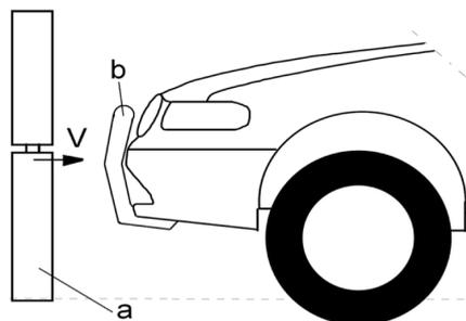
**Fig. 1.** Lower legform impact testing: a – legform impactor, b – frontal protection system, V – velocity of the impactor.
