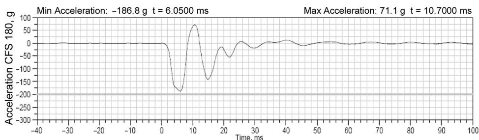
Fig. 3. Acceleration plot of the lower legform impact test.
