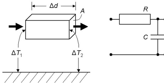
**Fig. 2.** Heat flux and related thermal RC network.
