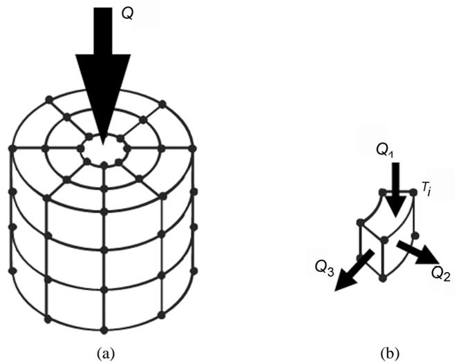
**Fig. 5.** Finite elements: a – division of the sample into small elements and direction of the excitation heat flux  $Q$ ; b – single element with its nodal temperature  $T_i$  and internal partial heat fluxes  $Q_j$ .
