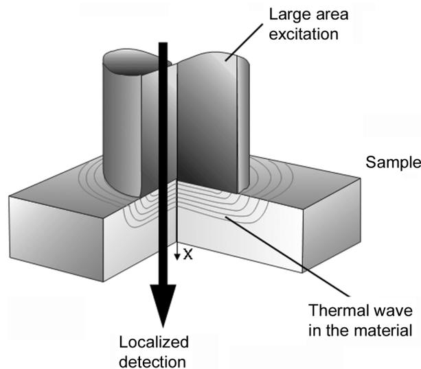
**Fig. 3.** Excitation and detection spots for plane thermal waves.
