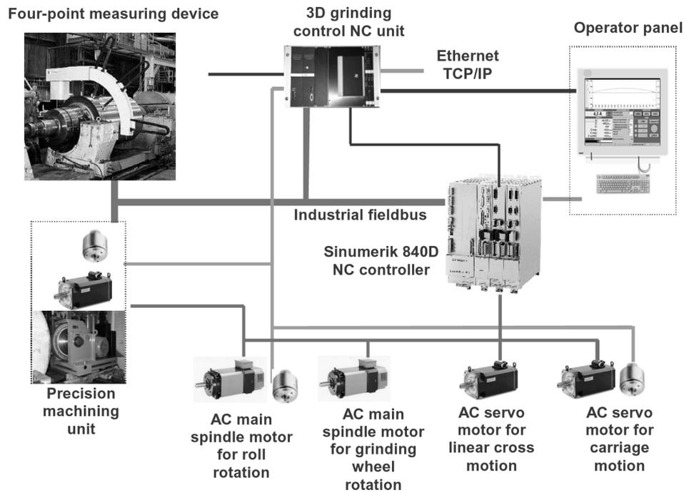
**Fig. 4.** Generic description of the 3D measuring and grinding system.
