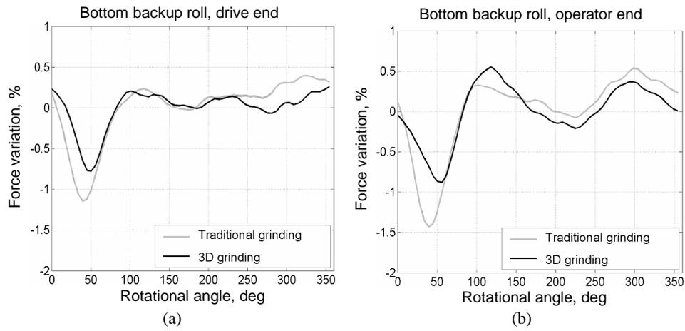
**Fig. 11.** Force variation caused by bottom backup roll after traditional grinding and 3D grinding at the drive side (a) and at the operating side (b).
