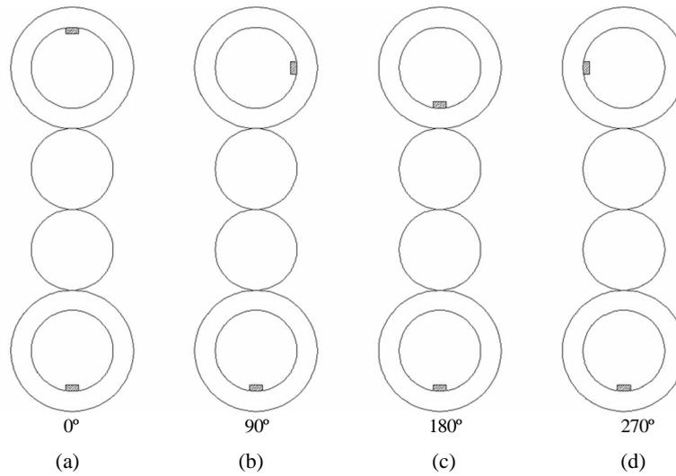
**Fig. 12.** Differences of the diameter of the backup rolls causes a relative phase shift of the key grooves; the roll force variation reaches its maximum, when both key grooves are under load at the same time, i.e. the relative groove positions are close to the situation as shown in (a).
