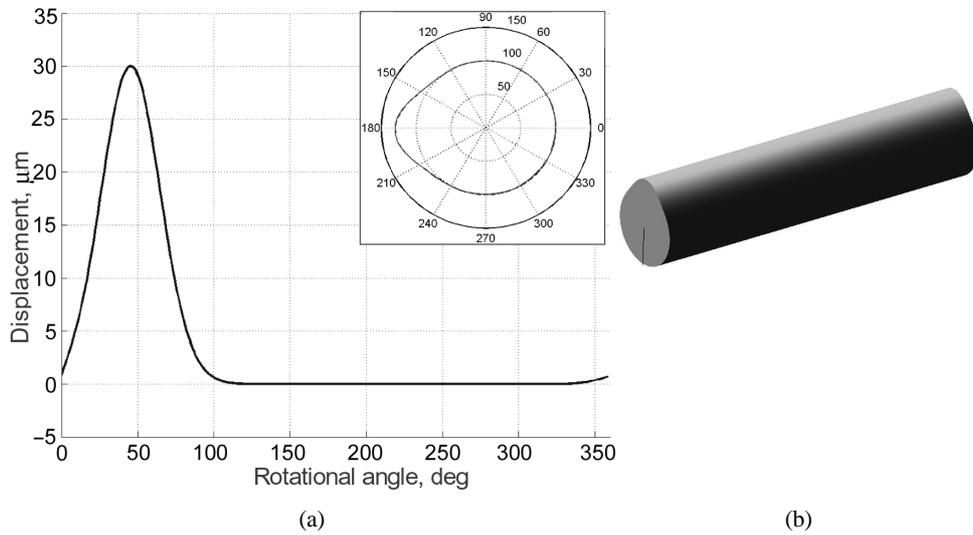
**Fig. 8.** (a) The calculated 30 μm 2D correction profile for each cross section of the roll; (b) the same profile applied to the whole length of the backup roll (not in scale).
